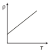
Resistivity as a function of temperature for alloys
